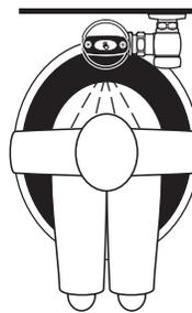
3. When the user steps away from the OPTIMA Plus Sensor, the circuit waits 3 seconds (to prevent false flushing) then initiates an electrical signal that operates the Solenoid. This initiates the flushing cycle to flush the fixture. The Circuit then automatically resets and is ready for the next user.
