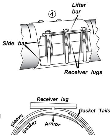
**Step 5** • Tighten all nuts evenly in 20 ft-lbs increments. Start tightening in the center of the clamp, working toward each end. Keep the torque as even as possible between all nuts. It is necessary to re-torque every nut several times (4-8) in order to maintain the proper torque. Start at 20 ft-lbs, then 40 ft-lbs, 60 ft-lbs, and finally 80 ft-lbs, or until the recommended torque has been reached. See table below. Use a wrench with at least a 12" handle.
