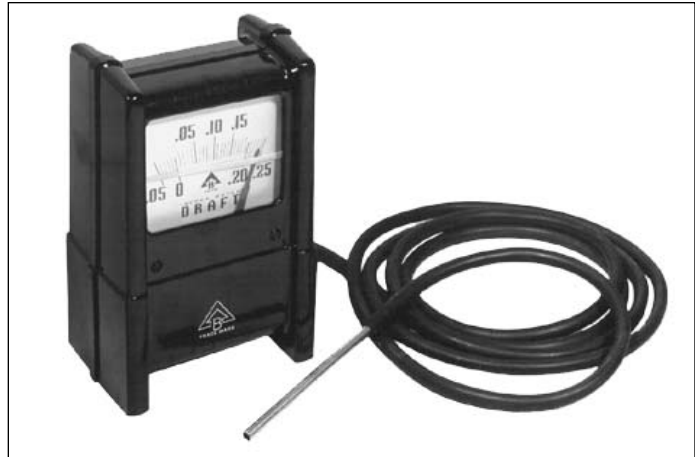
Figure 14.1 Draft Gauge with Probe
