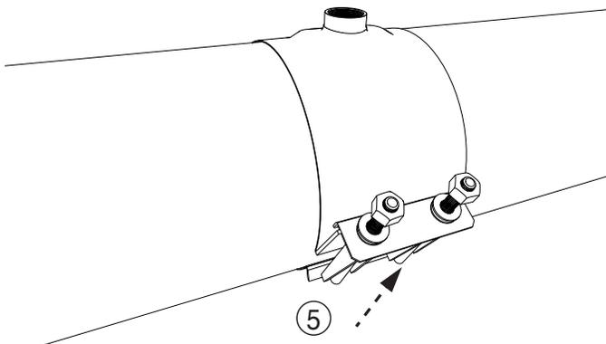
**Step 6** • Tighten all nuts evenly in 20 ft-lbs. increments. Use a wrench with at least a 12 inch handle. Close all gaps between the shell and the pipe surface evenly, and torque according to specifications below. Bolt resistance will increase quickly once the saddle is properly installed.
