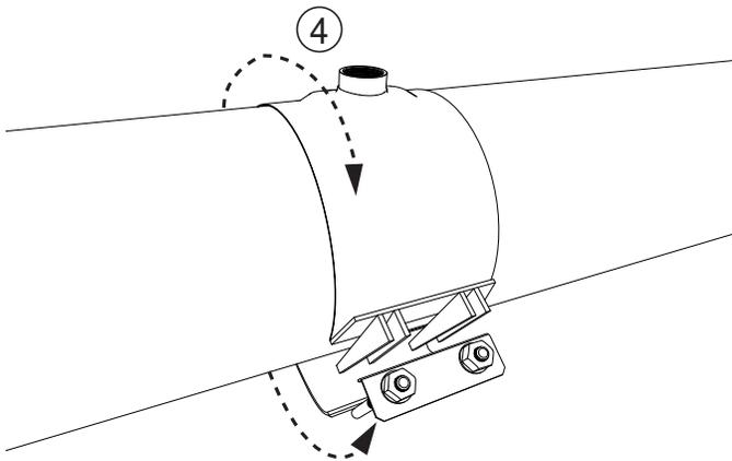
**Step 5** • Slide lifter bar up the receiver lug profile and snap into place over the sidebar edge. Confirm that the gasket is aligned in its pocket.
