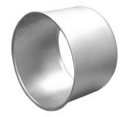
JCM HDPE Pipe Stiffeners are designed to support the interior wall of HDPE for critical pipe joining applications. Recommended for all pipe end connections utilizing mechanical bolt-on fittings, the JCM Pipe Stiffeners support the pipe's end and controls the "necking down" reaction to the pressure applied during normal installation of fittings used in pipe joining applications.
