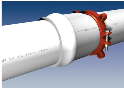
3. Install both halves of the serrated ring around the pipe behind the bell, tapping each half into place. Make sure that the complete ID of the ring is touching the pipe before installing the side bolts. Install the side bolts and tighten evenly to 110 ft-lbs. of torque. (60 ft-lbs on 4 inch and 6 inch)
