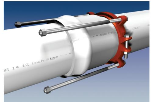
4. Remove the side bolts from the second serrated restraint ring. Use the Thrust Bolts to determine the proper location of the restraint ring on the spigot. Allow enough room on the thrust bolt to fully engage the nuts.
