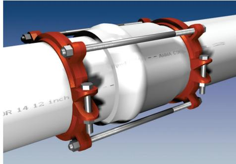
6. Place nuts on the thrust bolts and tighten until they are snug. Allow enough room on the thrust bolts to fully engage the nuts. Do not tighten these bolts enough to force the spigot further into the bell of the joint.
