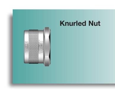
The knurled nut is used with fittings where applications of a finger tight assembly is acceptable. Common applications include, but are not limited to, low pressure laboratory use on plastic tubing.
