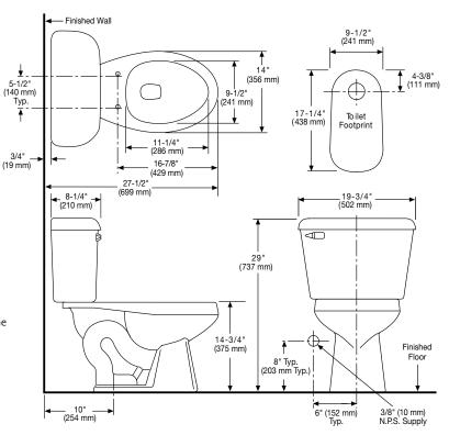
NOTE: Install this product according to the installation guide.
