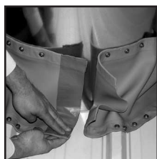
1. Cut splice tape to length, remove film from one side and apply to Dekstrip.
