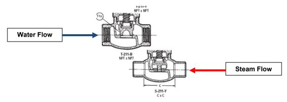
**For water service applications**: The flow should enter the valve so that it pushes up from underneath the seat disc. In other words, water flow should arrive from under the seat disc and flow smoothly out of the valve over the seat.
