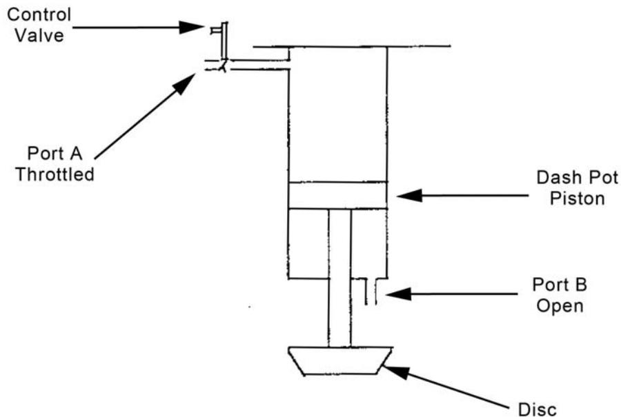
Now note that Port B is merely a drilled hole at the bottom of the dashpot, which allows the steam to enter and exit freely. Also, it serves to drain any resultant condensation. Port A, you will note, has a control valve which can be throttled to allow steam to enter the chamber above the piston, either rapidly for quick descent or slowly for a slow descent. This is a function of the
