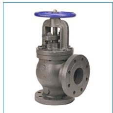
**Specifications UPC** Code 039923702036 Type Angle Valve **Valve Size** 6 **Connection Type** F -- Flanged Material Cast Iron Cv Coefficient 581.25 Standard Handwheel **Valve Operator Description** F869B 6 FLG ANGLE CAST IRON eClass Classification Stop-Check Cast Iron Check Valves **Turns/Operation** Non-Manual 311.006 lb Weight
