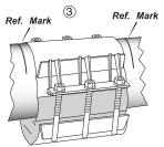
**Note:** If necessary because of flowing water, Steps 3 and 4 can be performed beside the pipe crack or hole. Slide the clamp over the break after the lifter bars have been snapped into place.
