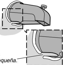
**6** Remove the excess sealant.
