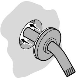
**11** Remove the excess sealant.
