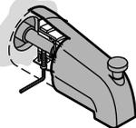
Overtightening may damage copper pipes!
