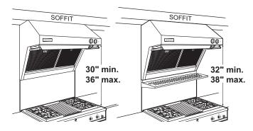
In this installation the ductwork running from the top of the hood will be concealed in the soffit or upper cabinetry.
