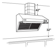
10 FT. CEILINGS When the hood is installed 36" above the cooking surface, order three 12" and one 6" duct cover accessories.
