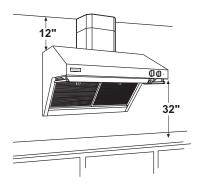
8 FT. CEILINGS When the hood is installed 32" above the cooking surface and there is no soffit or upper cabinetry, order one 12" and one 6" duct cover accessory.
