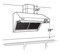
9 FT. CEILINGS When the hood is installed 38" above the cooking surface, order two 12" duct cover accessories.
