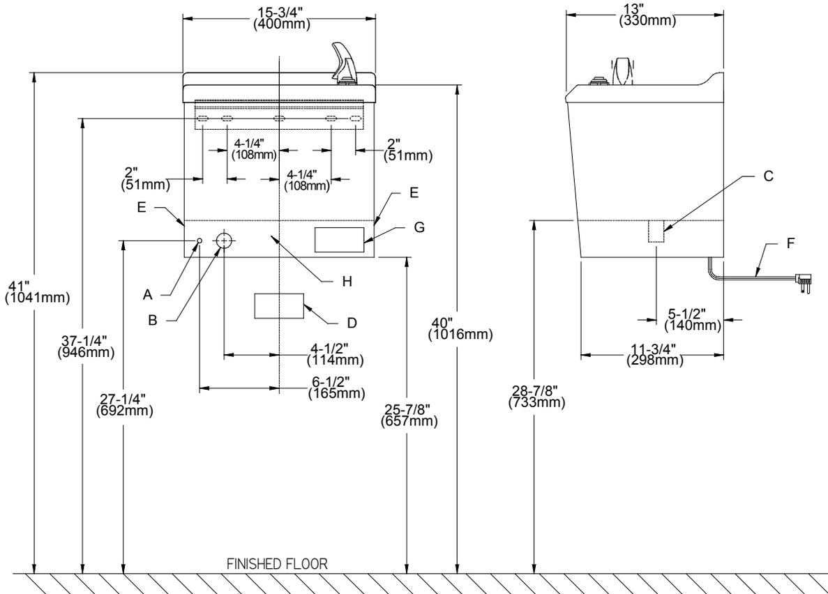
If recessed in an alcove, allow full opening beneath cooler, and at least 4" (102mm) or more on each side for air circulation.
