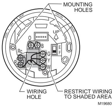
Fig. 5. Restrict T8775 wiring to shaded area.
