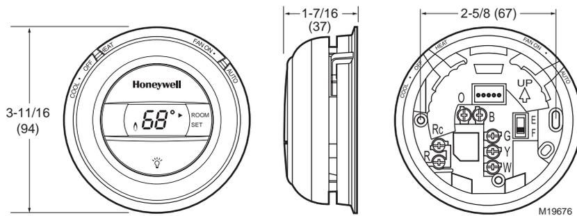
Fig. 1. T8775 Thermostat dimensions in in. (mm).
