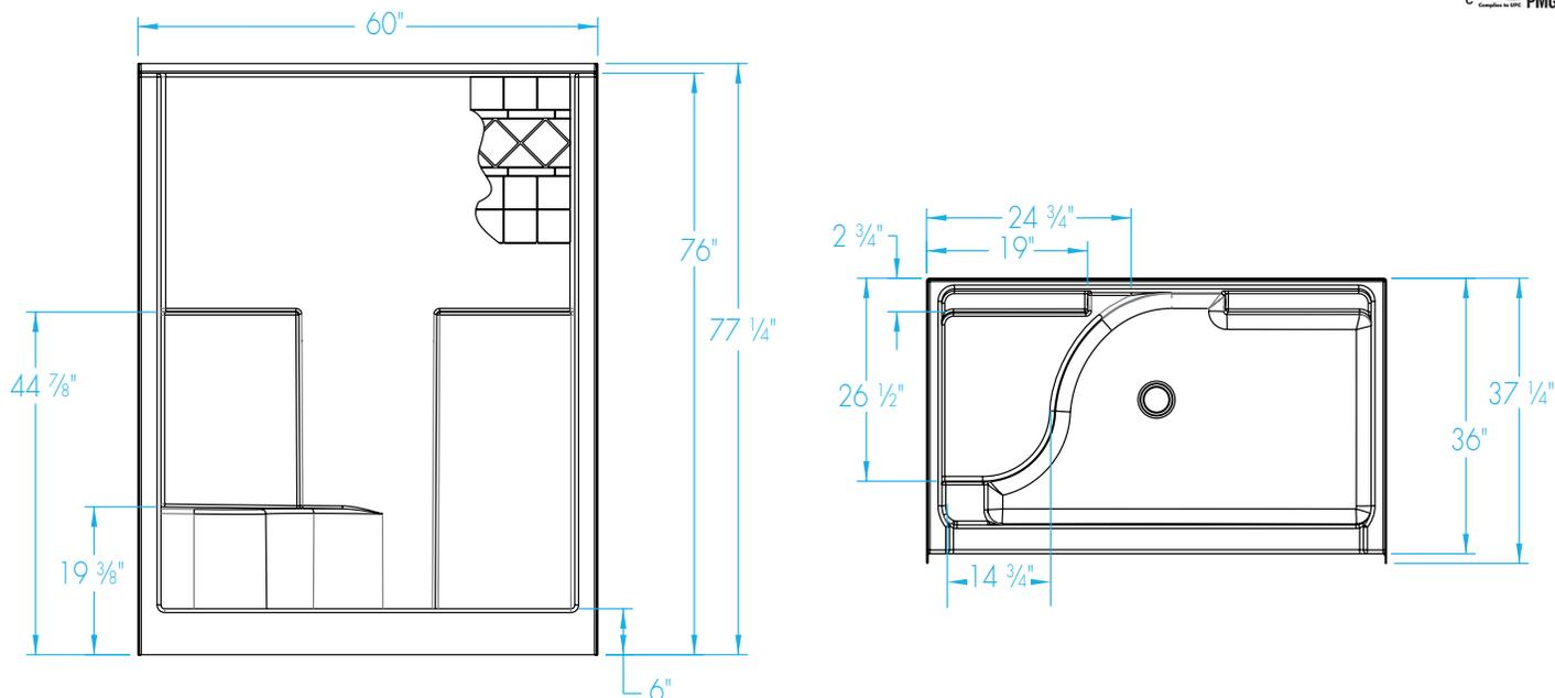
**FEATURES** lbs      Dimensional Tolerance  $\pm \frac{3}{8}$ ". Dimensions needed for site preparation should be measured from the unit. Aquatic assumes no responsibility for preparatory work.
