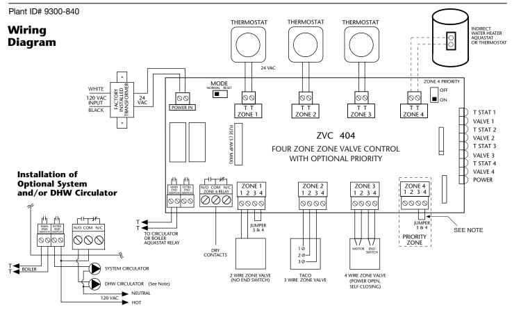
**Operation/External Diagnostics:** When any thermostat calls for heat, the appropriate zone valve is energized and the yellow light goes on. When the zone valve is fully open, the red light goes on and energizes the end switch relay. The green light should always be on, indicating that power is connected.
