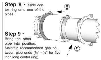
**Step 10** • The center ring should be centered such that the space between the OD of the pipe and the ID of the center ring is even all around the pipe. Slide gaskets into position with the beveled edge engaging the flared end of the center ring.
