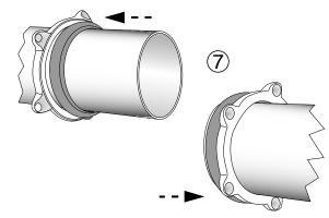
Note: Flexible Couplings do not provide protection against possible pullout of pipe ends in unrestrained conditions.
