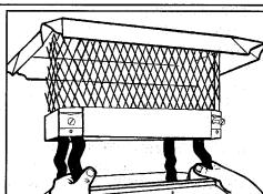
2. Insert two (2) legs into the liner no more than 1". By exerting pressure as shown, force the other legs inside the liner. Push cover straight down into the chimney liner as far as possible. Tighten the screws on all four (4) legs until the cover is held firmly into the Flue Tile.
