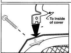
1. Slip the leg up through the lance inside each corner of the band until the hole in the leg is aligned with the hole in the lanced band. Insert the mounting screw (use same four screws enclosed with cover) through the hole in the leg and into the hole in the lance. Tighten the screws just enough to hold legs into the laced slots on each corner of the cover.
