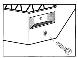
1. Insert one screw into the lower hole located in each mitered corner of the chimney cover band. (Just start the screw into the hole a few turns, until all four screws are started.)
