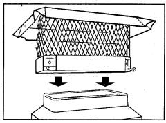
2. Place the chimney cover on the flue liner and align the base with the flue liner. Partially tighten each of the four (4) screws until they are snug to the liner. Then tighten each of the four (4) screws firmly to the liner.
