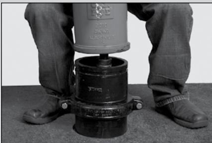
**6** Place Upper Standpipe on Extension, taking care to keep Standpipe Coupling Seal in place during assembly.
