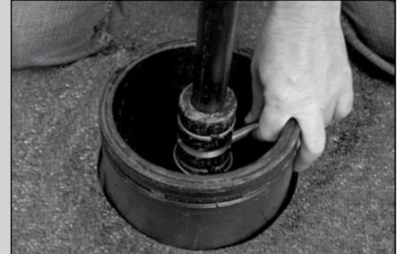
**2** Slide bottom Coupling Retaining Ring out of groove, remove bottom Rod Coupling Pin and separate Upper Valve Rod with Valve Rod Coupling still attached from Lower Valve Rod. Remove and save Dampener ring.
