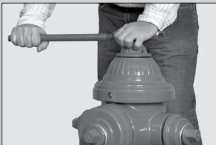
**5** Close the hydrant Main Valve first, then open the auxiliary hydrant control valve. Operate the hydrant and check for leaks.
