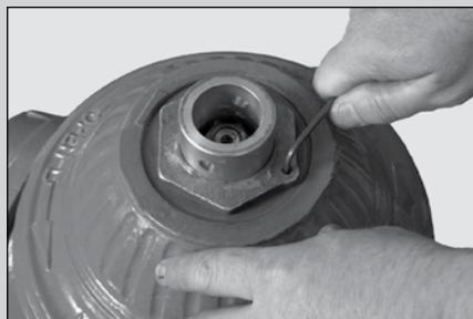
**8** Re-grease both upper and lower chambers of Revolving Nut. Then, reinstall Hold Down Nut and tighten securely. Install and tighten Hold Down Nut Screw, and finally reinstall Operating Nut and Operating Nut Locking Pin.
