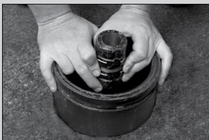
**4** Install new Valve Rod Coupling, and slip stainless steel Coupling Retaining Rings up and out of grooves, for Pin removal. Put replacement Valve Rod Coupling over top of Lower Valve Rod— make sure Dampener ring is in place inside coupling at top of Lower Valve Rod. Replace lower Pin and slip Coupling Retaining Ring down, snapping back into groove and locking Pin in place.
