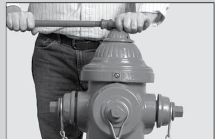
**8** Make sure operating parts are clean and well lubricated before reassembly. Reassemble Bonnet onto extended Valve Rod assembly, following steps 7, 8 & 9 of the disassembly/reassembly procedure on Page 7.
