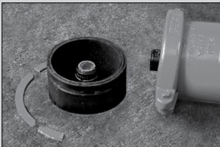
**2** If damaged, replace Standpipe Coupling Seal. Fill groove with grease to keep seal in place during assembly.
