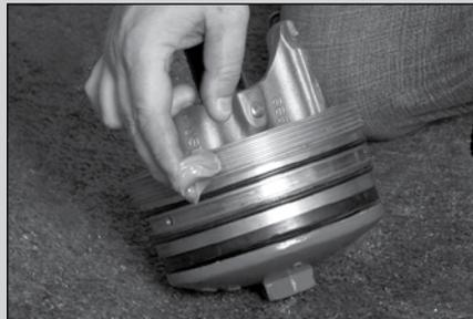
**5** Lay out all components, replacing worn, damaged ones as needed. Clean first, then grease all threaded parts, using a lubricant such as Diana 2100 (replacement grease must be compatible with calcium sulfonate grease). After lubrication, reassemble parts and securely tighten Bottom Valve Plate.
