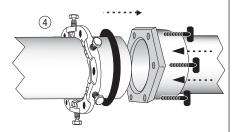
**Step 5** • Slide the gland toward the joint until the raised lip of the gland touches the gasket. Insert the T-bolts and hand tighten the nuts. Make any deflection adjustment after hand tightening the T-bolt nuts but before tightening them to the proper torque specifications (5° maximum).
