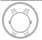
**Standard:** Assists installation and carries slip joint bells at least.75" off casing wall. Maintains dielectric insulation. No restraint against movement such as floatation or surge pressure bucking.
