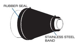
CASCADE Model CCES End Seals pull over the casing and carrier pipes after installation to provide a barrier to backfill debris and seepage.
