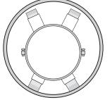
**Restrained:** Keeps carrier at bottom of casing while restraining against movement.
