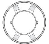
**Centered & Restrained:** Positions carrier in center of casing. Provides restraint against movement. Best for mechanically restrained pipe joints.
