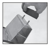
Cascade's Runners can be replaced in the field if bore is offgrade or installation is not to design.
