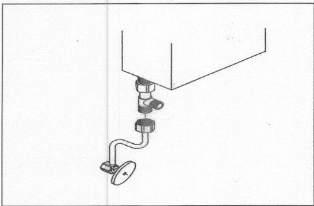
7. Connect Flexible water hose (provided) from T connector (1/2" threaded side) to system external water tank located under the control panel.
