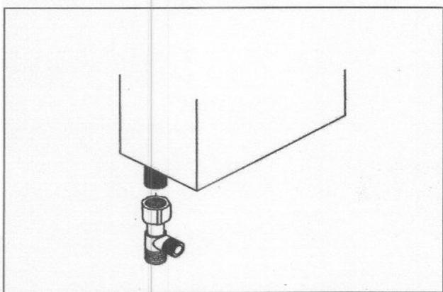
6. Connect water hose to T connector. (7/8" threaded side)
