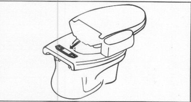
※ To Uninstall: push seat release button (see figure) and slide off the bidet unit.
