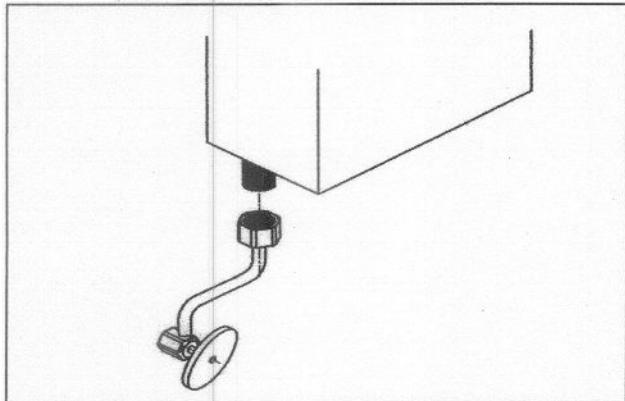
5. Attach T connector (provided) to the bottom of the water tank. Teflon tape is not required for installation. Keep all connections aligned and do not over tighten, as this may damage Connections.
