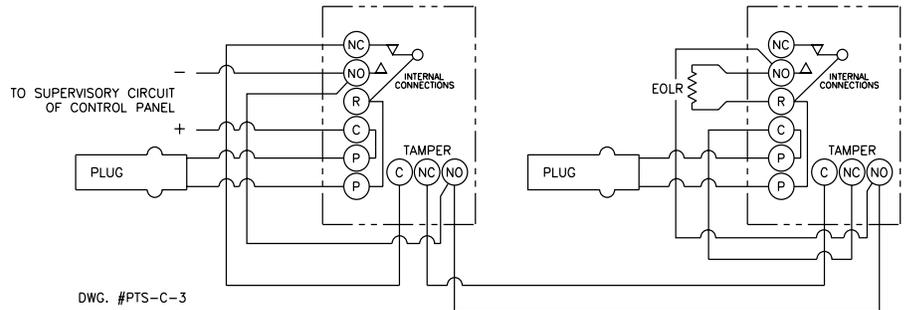
**Plug And Cover Tamper Wired To Separate Circuits**
