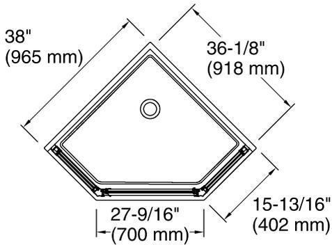
**Note:** Dimensions are taken on centerline of curb/threshold at the rough opening.
