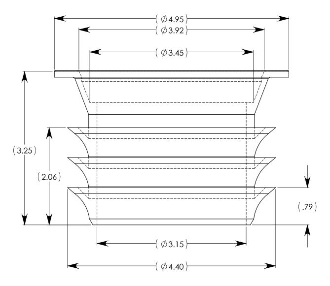
Gasket Material: Black Plasticized PVC 60 Shore A Durometer Hardness
