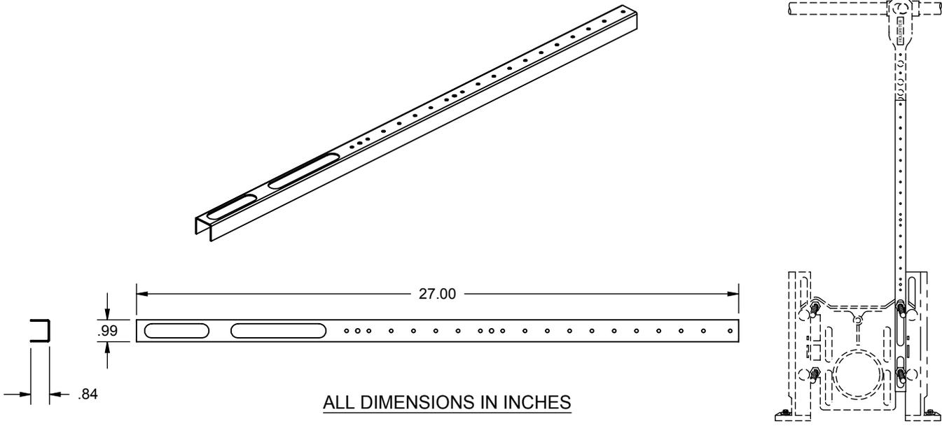
The HOLDRITE® #114-C-EXT is a Copper-Bonded™ steel bracket used to extend the flushometer rough-in height of the model #114-C, #114-CO and #114-CR an additional 8-1/2" through 24-1/2". The bracket mounts to the water closet carrier. Includes hardware for connection to the #114-C, #114-CO and #114-CR brackets.
