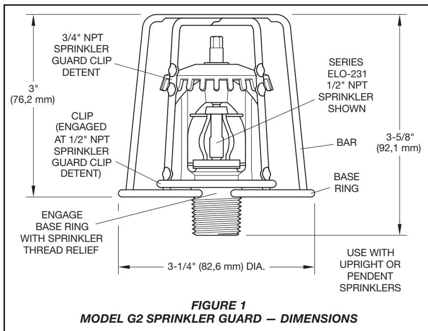
the “1/2 inch NPT Sprinkler Guard Clip Detents” or “3/4 inch NPT Sprinkler Guard Clip Detents”, as applicable, to complete the installation as shown in Figures 1 and 3.
