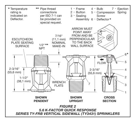
Automatic sprinklers must never be painted, plated, coated or otherwise altered after leaving the factory. Modified sprinklers must be replaced. Sprinklers that have been exposed to corrosive products of combustion, but have not operated, should be replaced if they cannot be completely cleaned by wiping the sprinkler with a cloth or by brushing it with a soft bristle brush.
