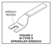
After installation, the sprinkler wrench flats and frame arms must be inspected and the wax coating retouched (repaired) whenever the coating has been damaged and bare metal is exposed. The wax coating on the wrench flats can be retouched by gently applying a heated 1/8 inch diameter steel rod to the areas of wax that have been damaged, to smooth it back over areas where bare metal is exposed.
