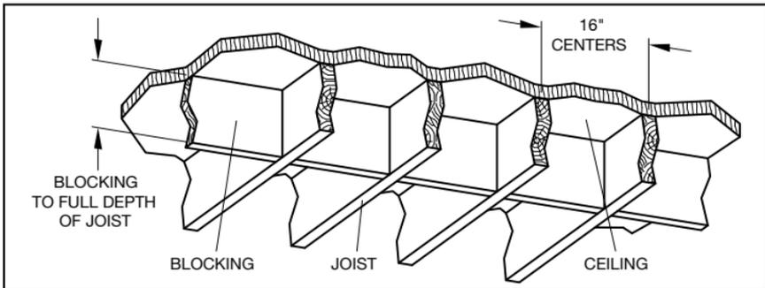
**Figure 5– Unfinished Basement, Branch Line Support**
