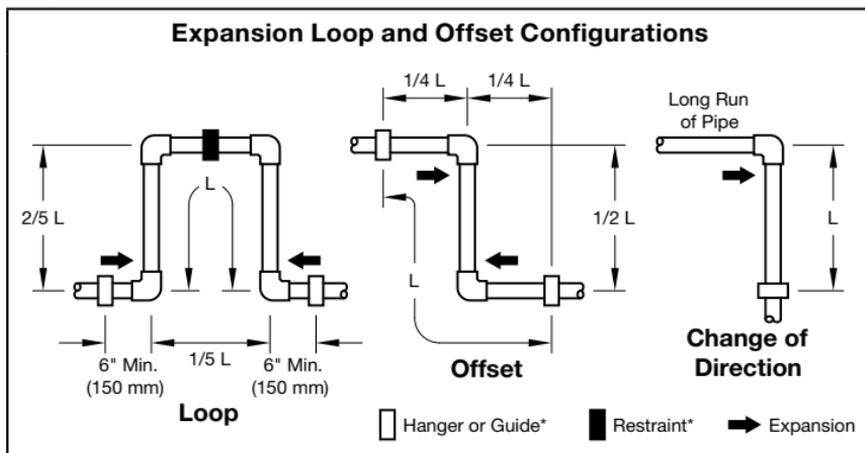
\* Hangers should only be placed in the loop, offset, or change of direction as indicated. Piping supports should restrict lateral movement and shall direct axial movement into the expansion loop.
