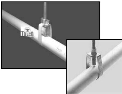
**Note:** Threaded rod shall not come in contact with CPVC when installed. It is advisable to use lift restraint devices such as those produced by Tolco and Afcon that prevent the threaded rod from coming in contact with the CPVC pipe (as shown above).
