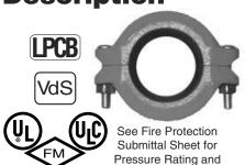
The Figure 716 Flexible Reducing Coupling allows a direct transition between two different pipe sizes, and replaces two couplings and a reducing fitting. It is capable of pressures up to 350 psig (2413 kPa) depending on pipe size and wall thickness when used in fire protection services. Note: Reducing Couplings are not recommended for dry pipe and freezer applications.
