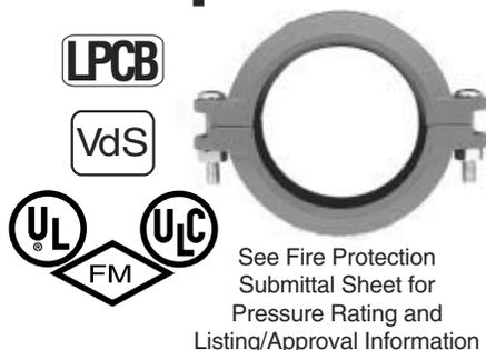
The Figure 772 Rigid Coupling provides a rigid joint by firmly gripping along the circumference of the pipe grooves. Rigid couplings are preferred for dry pipe and freezer applications. Figure 772 Rigid Couplings are a proven dependable method of joining pipe and are an economical alternative to welding, threading or using flanges. It is capable of pressures up to 500 psig (3447 kPa) depending on pipe size and wall thickness when used in fire protection services.
