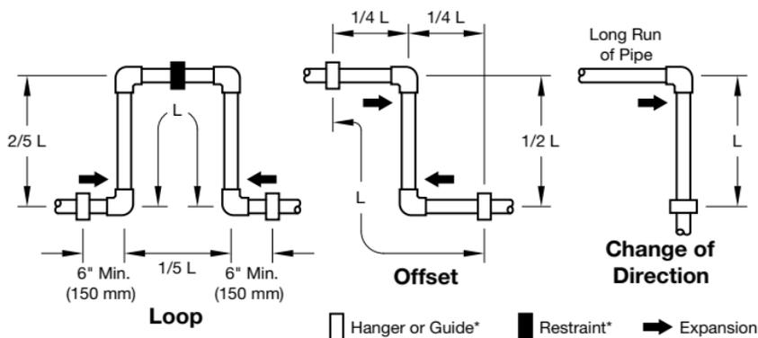
\* Hangers should only be placed in the loop, offset, or change of direction as indicated. Piping supports should restrict lateral movement and shall direct axial movement into the expansion loop.
