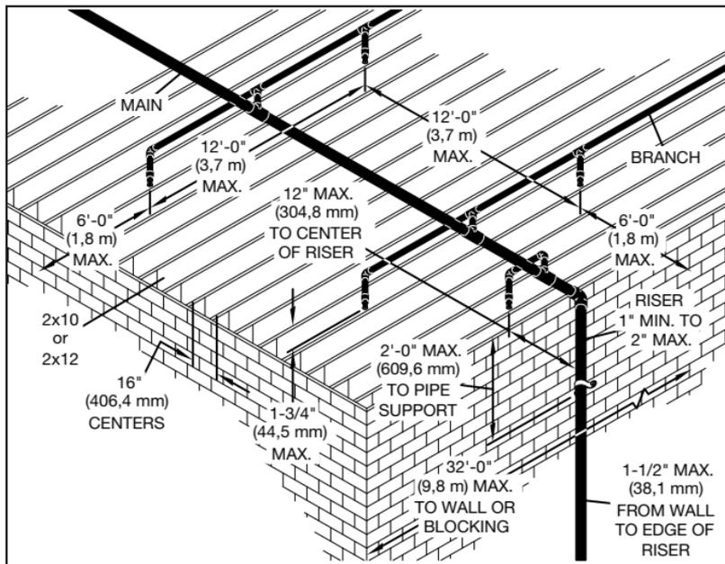
Figure 2 – Unfinished Basement, Center Wall Riser with Main at Wall
