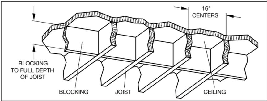
**Figure 5– Unfinished Basement, Branch Line Support**
