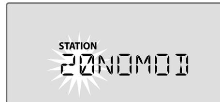
The screen displays “20NOMOD” with the “20” flashing to indicate that Station 20 (and also 21-22) are unused and unavailable for programming.
