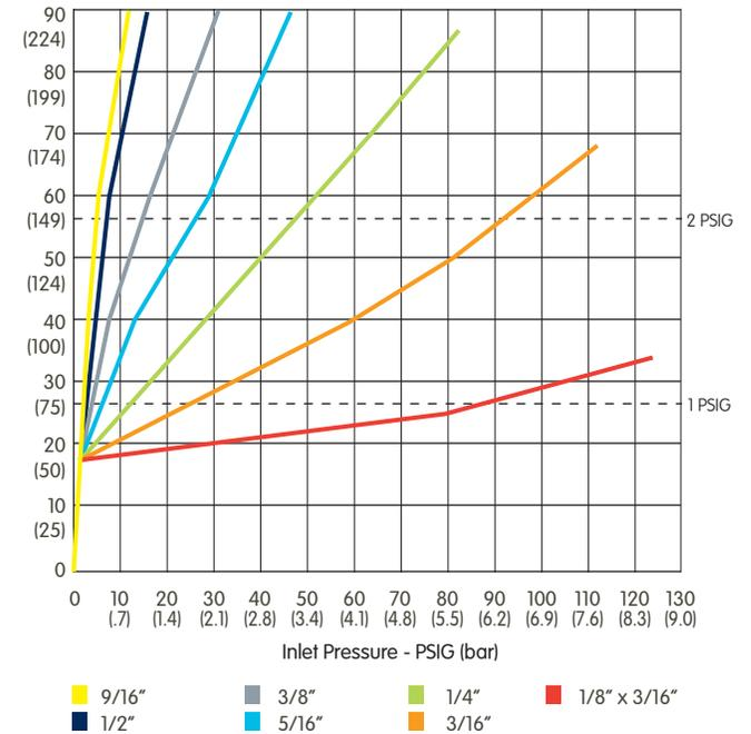
3/4" Screened Vent – No Vent Pipe Set Pressure 2 PSIG
