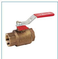
**Specifications UPC** Code 039923675446 Ball Valve Type **Valve Size** 2 T -- Female NPT Thread (FIPT) **Connection Type** Material **Bronze Ball Material** Brass with Hard Chrome Plate Stem Material Silicon Bronze **Valve Operator** CS Standard Lever Handle **Description** KT58070UL 2 UL W/LEV HDLE **Turns/Operation** Quarter-Turn Weight 5.092 lb
