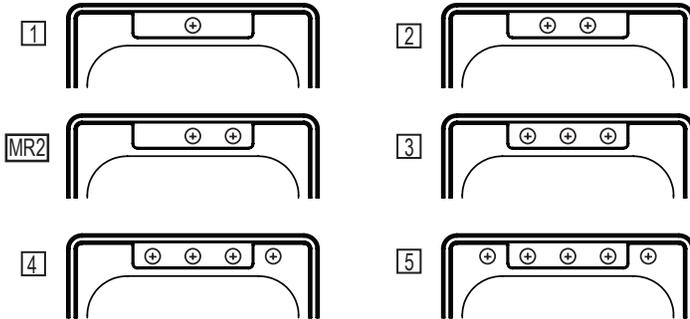
**Hole Drilling Configurations**
