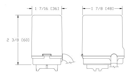
**Engineering Specifications:** Zurn 4 Wire Zone Valve Actuator allowing for individual zone control of QickZone® and AccuFlow® Heating Manifold. Unit operates on 24V AC, 3W. End switch is rated at 1.5A. Complete with pop up operating indicator, integral end switch, and snap on/off manifold attachment. Unit operates up to a maximum ambient air temperature of 122° F (50°C).
