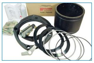
A hydrant so low that connection of a hose is impossible or difficult is a community hazard. The Waterous Top Extension Kit allows for fast and inexpensive extension of the nozzle section, to any desired height (in 6" increments) in case of grade change.
