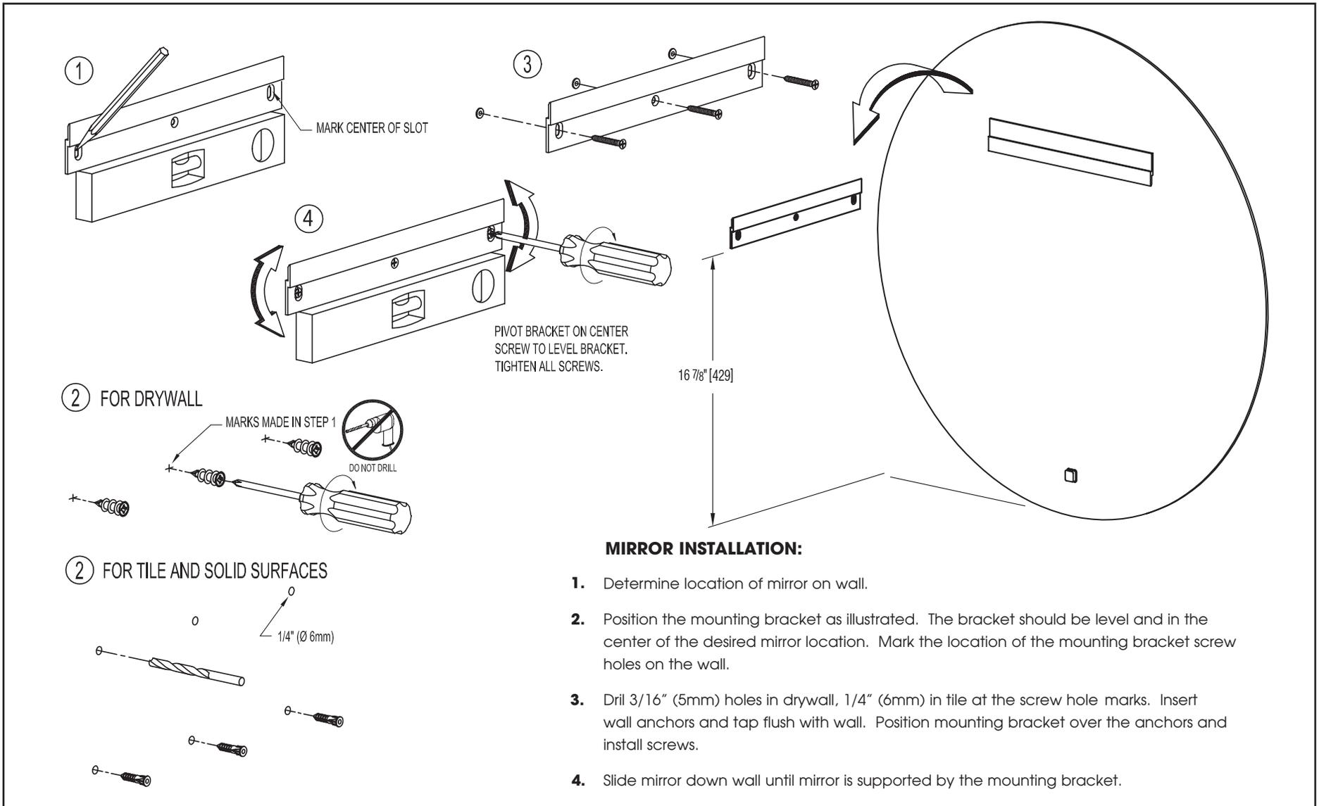
**Tools needed:** Pencil, Tape measure, Phillips Screwdriver, Drill and Level.
