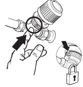
If required firmly press anti-theft lock into inner ring to prevent unauthorised removal
