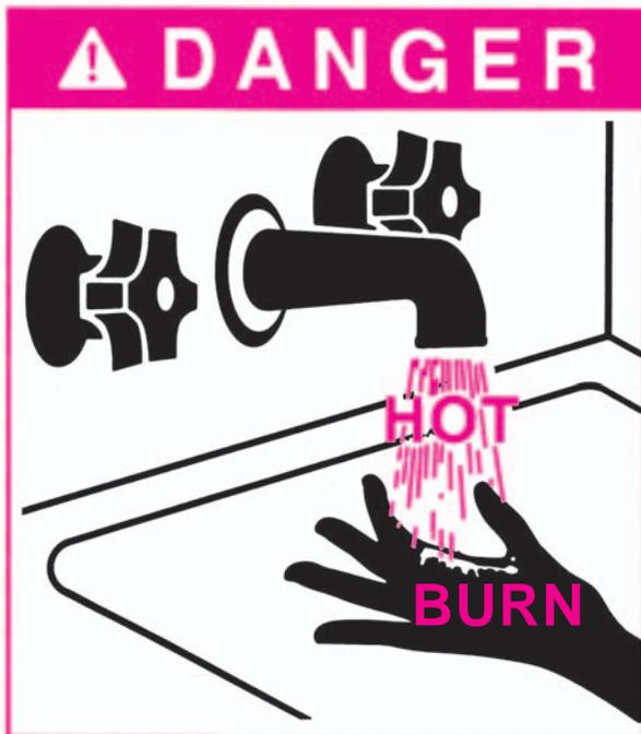
Water Temperatures over 125°F can cause severe burns instantly or death from scalds.
