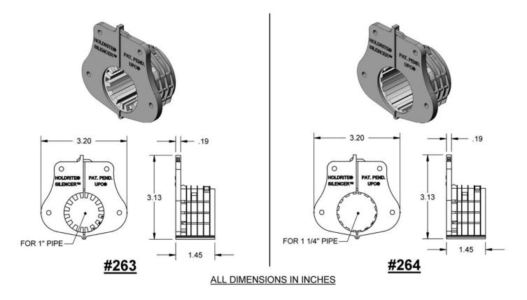
Model #'s 263 and 264 can be used as a suspension hanger, e.g., from a joist or cross-member or a Holdrite<sup>®</sup> Stout Bracket, or as a through-hole isolator in wood or metal framing. As a through-hole isolator, mounts in 2" hole in wood or sheet metal up to 14 gage. Secures and retains tubing while providing superior acoustical isolation between the tubing and the supporting structure. Supports 1" and 1-1/4" CTS tube sizes. Supports Copper, PEX and CPVC tubing.
