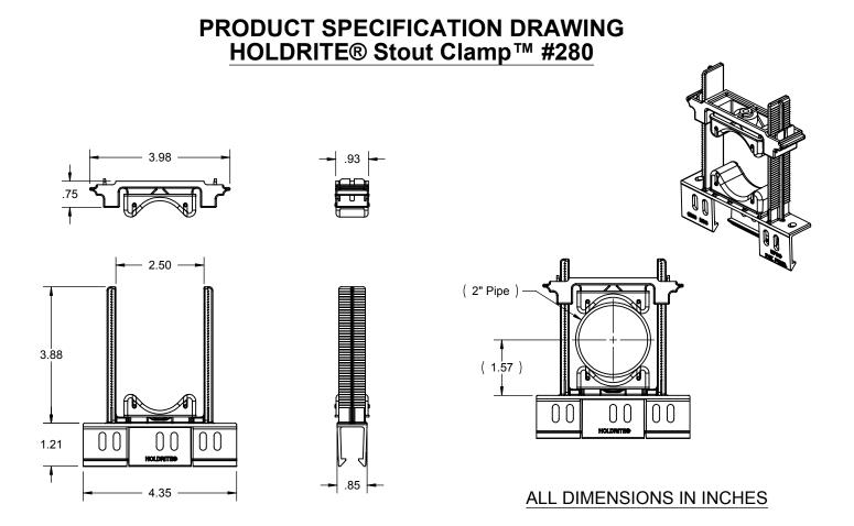
Sound rated variable closure clamp that may be installed to HOLDRITE® EZ-Strut™ or Stout Brackets™ with only one to three screws (for maximum load in suspension mode). Two acoustical inserts isolate the pipe from the supporting structure, reducing waterline noise and vibration, while allowing normal pipe expansion and contraction. Variable closure clamp supports 1" - 2" CTS and IPS pipe sizes. Supports Copper, PEX, CPVC tubing, conduit, etc. Frame complies with UL94V-2 frame rating.
