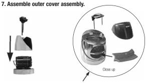
Note. Verify that rubber insert is installed
