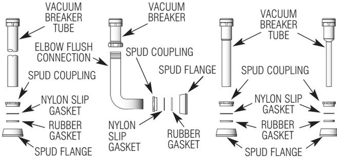
**B** Insert Tube into Fixture Spud.
