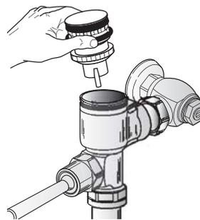
**C** Install Flushometer Cover wrench tight. Open Control Stop to flush supply line. Close Control Stop and remove Flushometer Cover.
