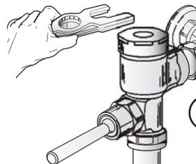
**D** Reinstall Piston Assembly and Flushometer Cover. Tighten Flushometer Cover wrench tight.
